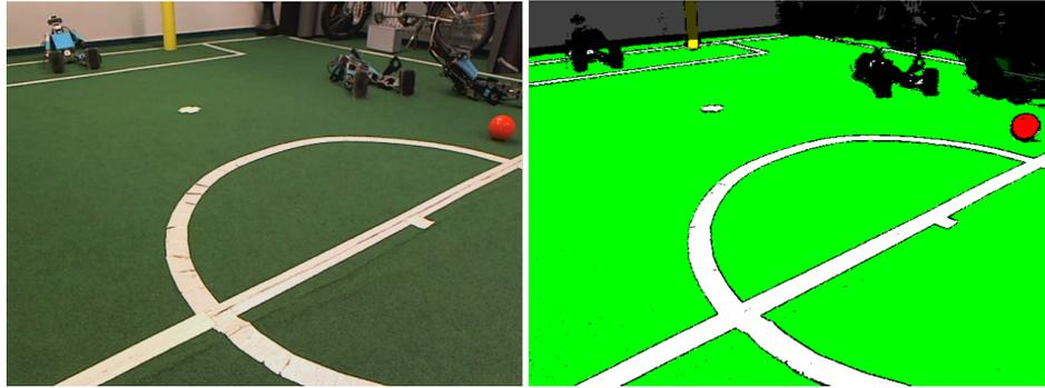
(a) Typical camera output (b) The classifier differentiates between the logical colors *ball*, *field*, *field line*, *goal* and *unknown*
