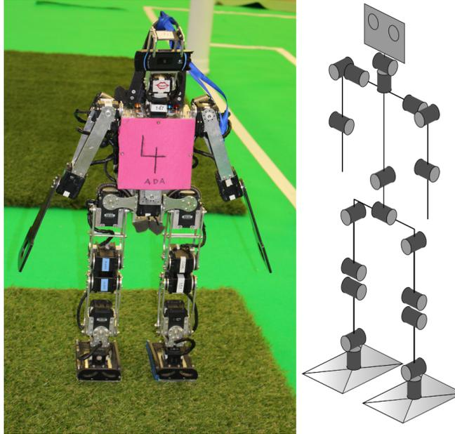
Fig. 1: Current model (left) and its kinematics (right)
