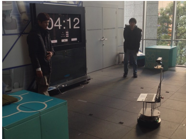
Fig. 5. Vision system on top of the robot
