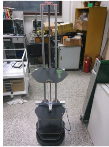
Fig. 4. Elevated platform for flexible height manipulation
